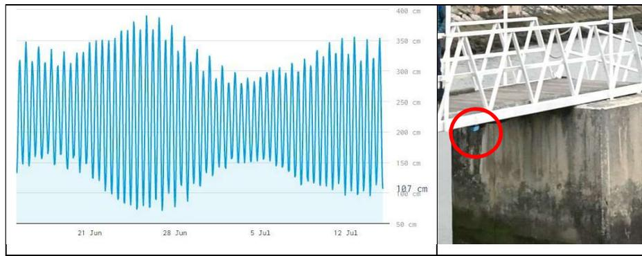
87 **Fig. 1.** Real-time sensor: a) elevation time series b) sensor location in the Marina (red mark).
