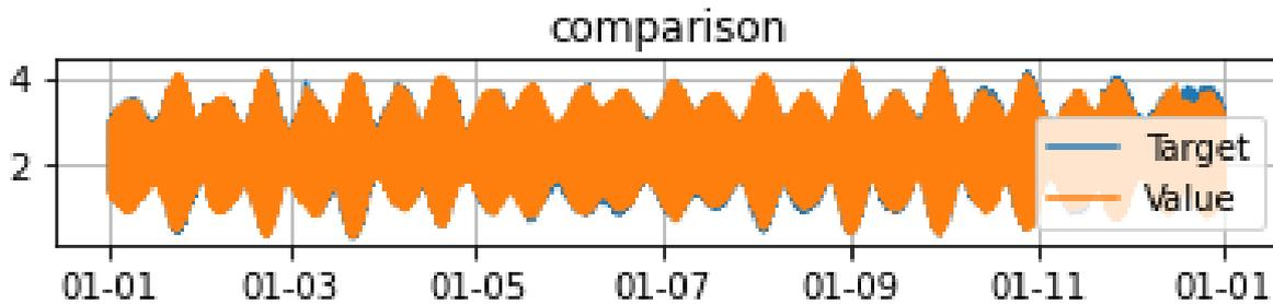
FIGURE 4 – Comparison of the water level computation with in-situ tide gauge with inverted barometer.
