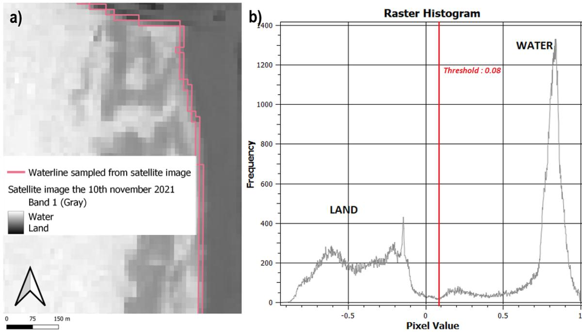
FIGURE 2 – Waterline (a) computed with the auto NDWI threshold (b)
