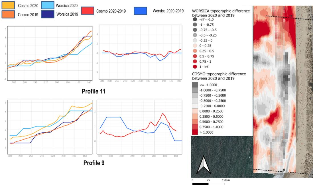
FIGURE 6 – Beach profiles (left) and their evolution (center). On the right, a map displaying the morphological evolution using COSMO overlapped by WORSICA evolution DTM values between 2019 and 2020. Profile 9 down, profile 11 top.
