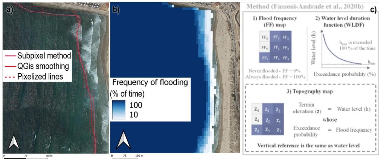
FIGURE 3 – a) The 3 ways of computing a waterline; b) Flooding frequency map in percentage of time a pixel is flooded; c) Explanation of the flooding frequency method.
