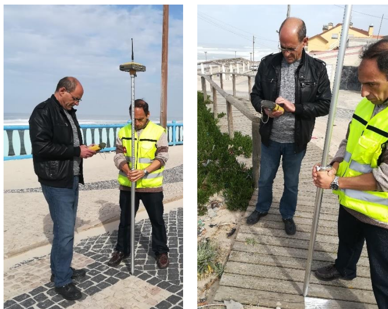
Figure 6.5 – Coordination of two points by GNSS-RTK in Vieira beach on 27/Feb/2019
